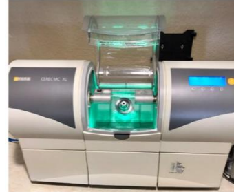
The milling machine used to make crowns using CAD/CAM technology.
